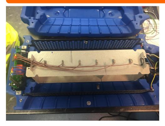
Product opens up into two sections with the base coming away to reveal all of the internal in one half of the shell.
